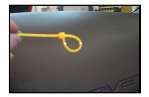
Remove the factory bulbs. (careful, they may still be hot). A little trick we like to use is using a small plastic wire tie to slip around the base of the bulb, pull it tight and pull the bulb out. Avoid using anything metal to remove them as you may short out the contacts.
